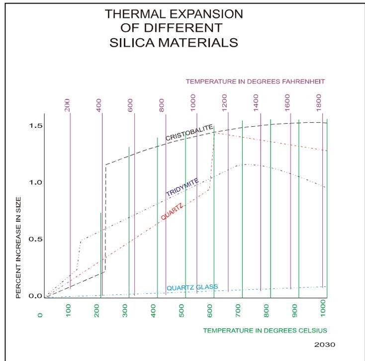
As the Starbars go through these temperature ranges, the expansion and contracting of the silica can fracture the silicon carbide lattice structure which increases the electrical resistance and can cause element failure.
